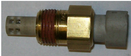
Open-element sensor suitable for air temperature.
