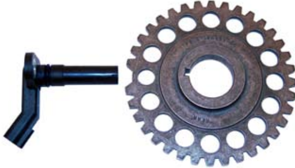
Typical 36-1 crankshaft position wheel and sensor, as found in many Ford engines
